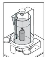
Once the necessary weights have been determined, the density of the Liquid sample is displayed in **g/cm<sup>3</sup>** (along with the weight in air, weight in water) on the Application screen.
