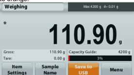
**Notes**: The first time a USB flash drive is connected to the balance there might be some delay time before the button **Save to USB** works. This is due to that the balance is creating the necessary folders on the USB flash drive where the data will be stored.
