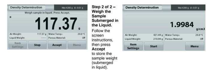
Once the necessary weights have been determined, the density of the sample is displayed in  $g/cm^3$  (along with the weight in air, weight in water) on the Application screen.
