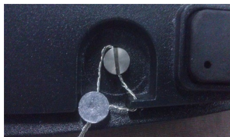
Locked with Wire Seal
